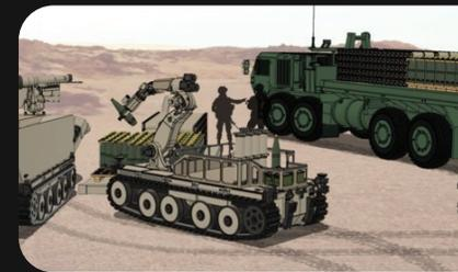
**EMV++ //** The EMV from Pratt Miller will be outfitted with an Aptronik robotic arm and custom applique kits to autonomously support larger as well as heavier projectile charge sets and increase rounds fired per day.
