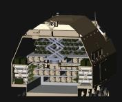
FUZE-SETTER // CR Tactical developed an automated fuzing system that removes the shipping lug from a shell, inspects the fuze well, manipulates a secondary charge (if present), and properly installs a fuze.
