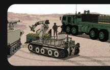
**EMAV++** // The EMAV from Pratt Miller will be outfitted with an Apptronik robotic arm and custom applique kits to autonomously support larger as well as heavier projectile charge sets and increase rounds fired per day.
