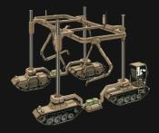
GANRTY // This deployable robotic unpacking station can process Class V supply into individual items by stripping away dunnage and packing material. It was designed by CR Tactical and features robotic arms from Apptronik.
